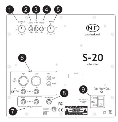
increase power handling. Setting the Subwoofer Bypass switch to BYPASS eliminates this circuit and sends all frequencies in the signal to the satellite monitors.
